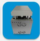
The YAX unit allows displacement of tools in lathe Y-direction, in order to produce manifolds where out-of-axis operations are required, such as face millings, holes and tappings, key-slots and so on. It can be fit on flat bed lathes as well as on slant bed lathes, where required y-axis movement is perpendicular to machine slide.
