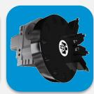
TB type turrets rotate thanks to a BRUSHLESS SER- VO-MOTOR, controlled by a new generation drive. Thanks to this new combination, extremely reduced times and shockless positionings are performed. Turret locking is achieved by means of belleville washers, ensuring high stiffness and safety.
